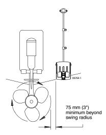
Figure 2-7: Mounting Location on Single Drive Boat
